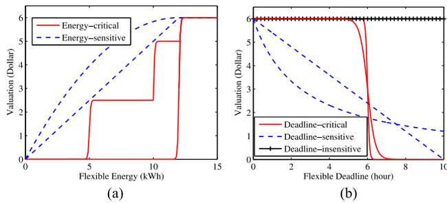
Fig. 1. Illustration of valuation functions of the flexible energy and deadline. (a) Energy-flexibility. (b) Deadline-flexibility.
