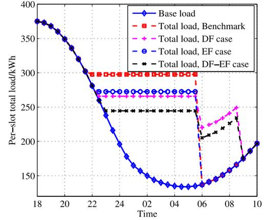
Fig. 2. Illustrating the valley-filling profile with different levels of flexibilities.
